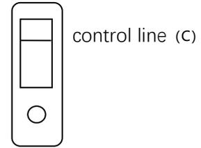
3. Invalid result: No ribbon appears on the control line (C). Invalid result is judged whether the detection line (G) (M) shows the ribbon or not. As shown in the figure.
