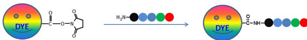
Figure 4.1. The reaction scheme of an amino-modified oligonucleotide with a dye succinimidyl ester.
