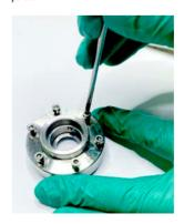
Do not screw completely. Leave a space of 1 mm between both parts to deal with thermal dilation during autoclaving.
