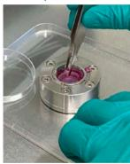
Screw with the clamping holder nut.
