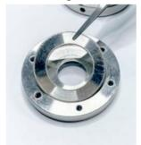
first and then the blade wedge washer on it. If you are using a 22 mm coverslip, place the blade wedge washer first and then the coverslip on it.
